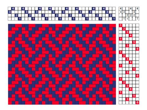
On four shafts, there are two twill lines that intersect two other twill lines going in the opposite direction; this forms the plait as can be seen in the drawdown on the left and the fabric below.
